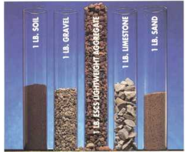
LWA offers more than twice the volume for the same weight of conventional aggregates.
