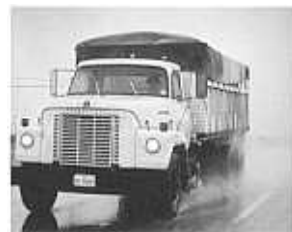
Hazardous truck spray and splash from regular dense-graded surface.
