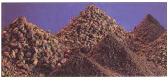
From a fiery rotary kiln comes lightweight aggregate processed in varying gradations and textures.
